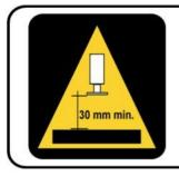
The space required between the support and the floor in the vertical position is 30 mm.
