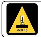
Use fixing points with sufficient stability. Consider every jack can lift up to 2500 kg. If necessary, the mounting points of the chassis must be reinforced with the correct parts.
