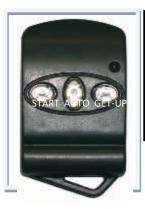
The main functions can be operated outside with the remote control. So, you have eye contact to the working of the jacks. You can control the floor conditions and set jackpads. Only the functions START – AUTO – GET-UP are available, other functions must be operated via the control panel.
