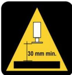
The space required between the support and the floor in the vertical position is 30 mm.
