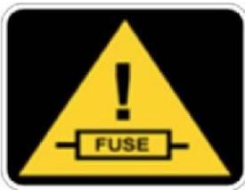
**When connecting to the battery, be sure to use the supplied fuse to avoid damage to the vehicle and the jacks. Insert the fuse into the + 12V / red cable**
