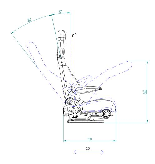
NB : THE DRAWING SHOWS THE SEAT WITH SWIVEL- AND SEAT INCLINATION-MECHANISM
