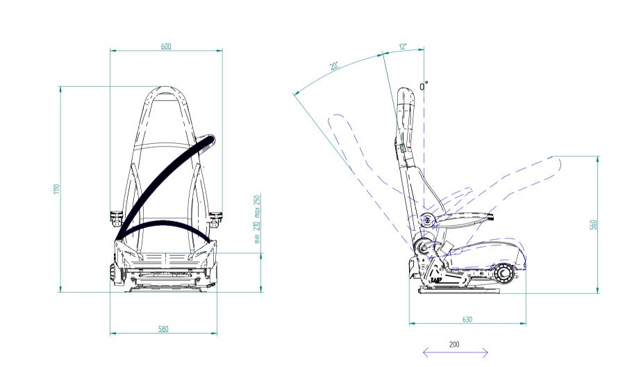
NB THE DRAWING SHOWS THE SEAT W/SWIVEL- AND SEAT-INCLINATION-MECHANISM SUITABLE FOR DUCATO X250 / PEUGEOT / CITROEN
